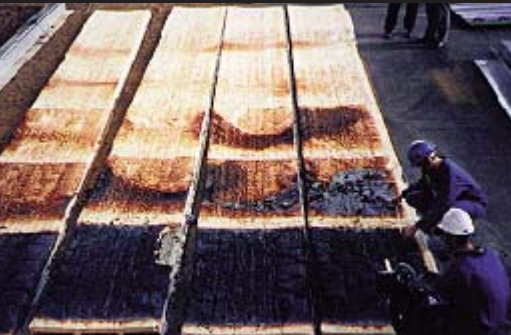
No spread of flame through the core between facings
