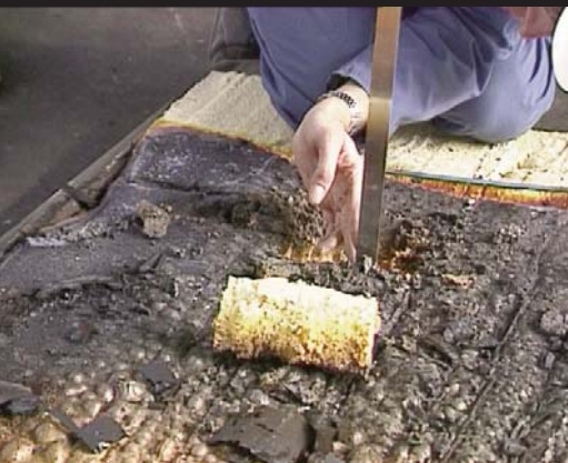
Stable protective char formed
