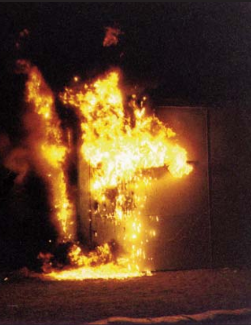
Polystyrene insulated panels External view during test
