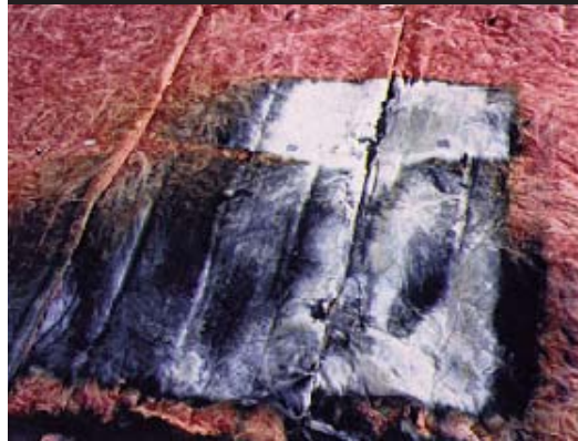
Shrinkage of glass fibre quilt from 86 to 20mm. (600°C) Insulation performance reduced
