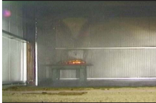
Sprinkler action: Panel damage significantly reduced
