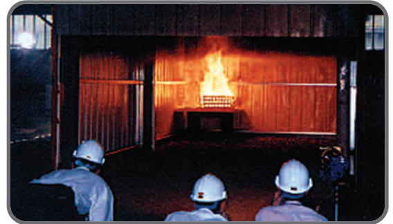
“Observation & recording – The tests generate an average heat output of 510KW and a max output of 1MW sufficient to represent a fire in the later stages of development”
