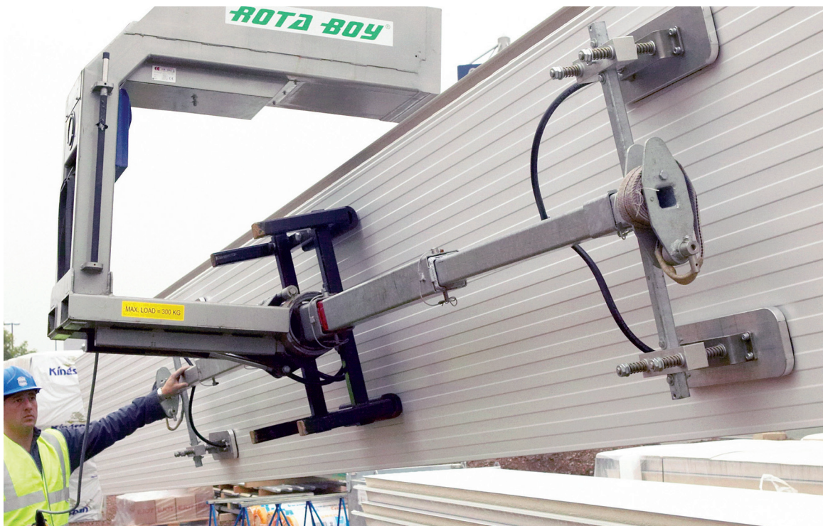
Example of handling and working with wall panels from ground level.
